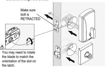
Before installing interior chassis, you will need to use a screwdriver to rotate the upper cam vertically as shown below to make mounting screw holes visible.
