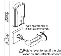
⚠Rotate lever to test if the plain latch extends and retracts smoothly. If not adjust mounting screws.
