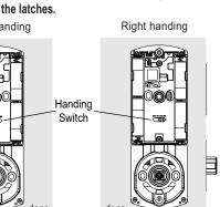
Flip interior chassis over. To change the handing of the spindle, pull out and then rotate.
