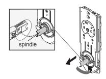
Install exterior assembly. Route cable underneath the latch bolt and through the shield.
