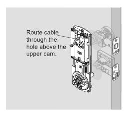
Make sure the flat blade is centered in the upper cam, and the spindle is engaged with the latch.
